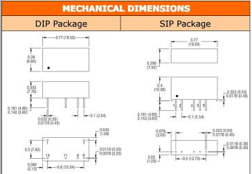
All dimensions in inches ±0.01(mm±0.25mm).All pins on a 0.1(2.54) pitch and within ±0.01(0.25)of true position.
