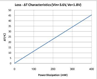
The output current of the device may need to be de-rated if it is operated in a high ambient temperature or in a continuous power delivering application. The amount of current de-rating is highly dependent on the environmental thermal conditions, i.e. PCB design, nearby components or effective air flows. Care should especially be taken in applications where the device temperature exceeds 85°C.
