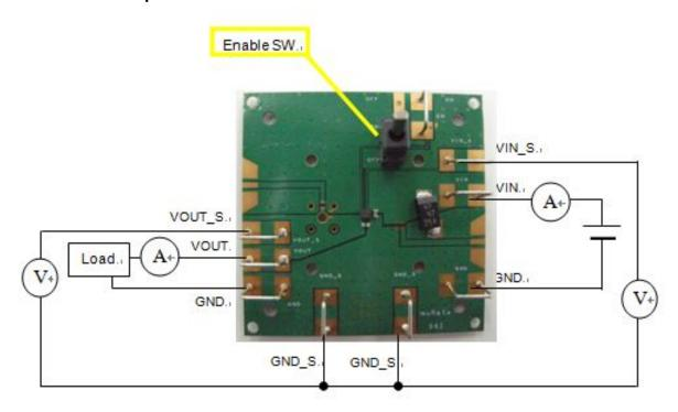
The enable switch has three positions.
