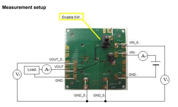
The enable switch has three positions.
