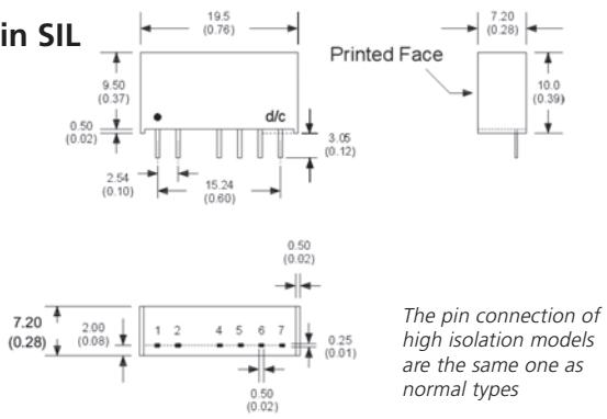
The pin connection of high isolation models are the same one as normal types
