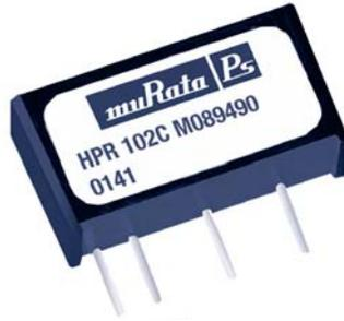
The HPR1XXC Series uses advanced circuit design and packaging technology to deliver superior reliability and performance. A 170kHz push-pull oscillator is used in the input stage. Beat-frequency oscillation problems are reduced when using the HPR1XXC Series with high frequency isolation amplifiers.
